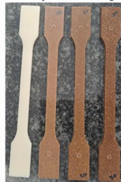
Injection moulded bio-composites and bio-composite films containing 0, 10, 20, 30 % cowpea lignocellulosic sidestream (from left to right)
